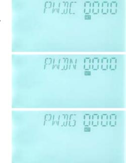
▶ Press SET button, "PWDG 0000" displays on the screen, ask for reentering the new password, doing like above to eenter the new password, "PWOK" displays on the screen to indicate reentering password successfully.
