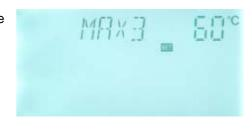
▶Press button to exit the menu or wait for 20 seconds to exit automatically, parameters are saved automatically.
